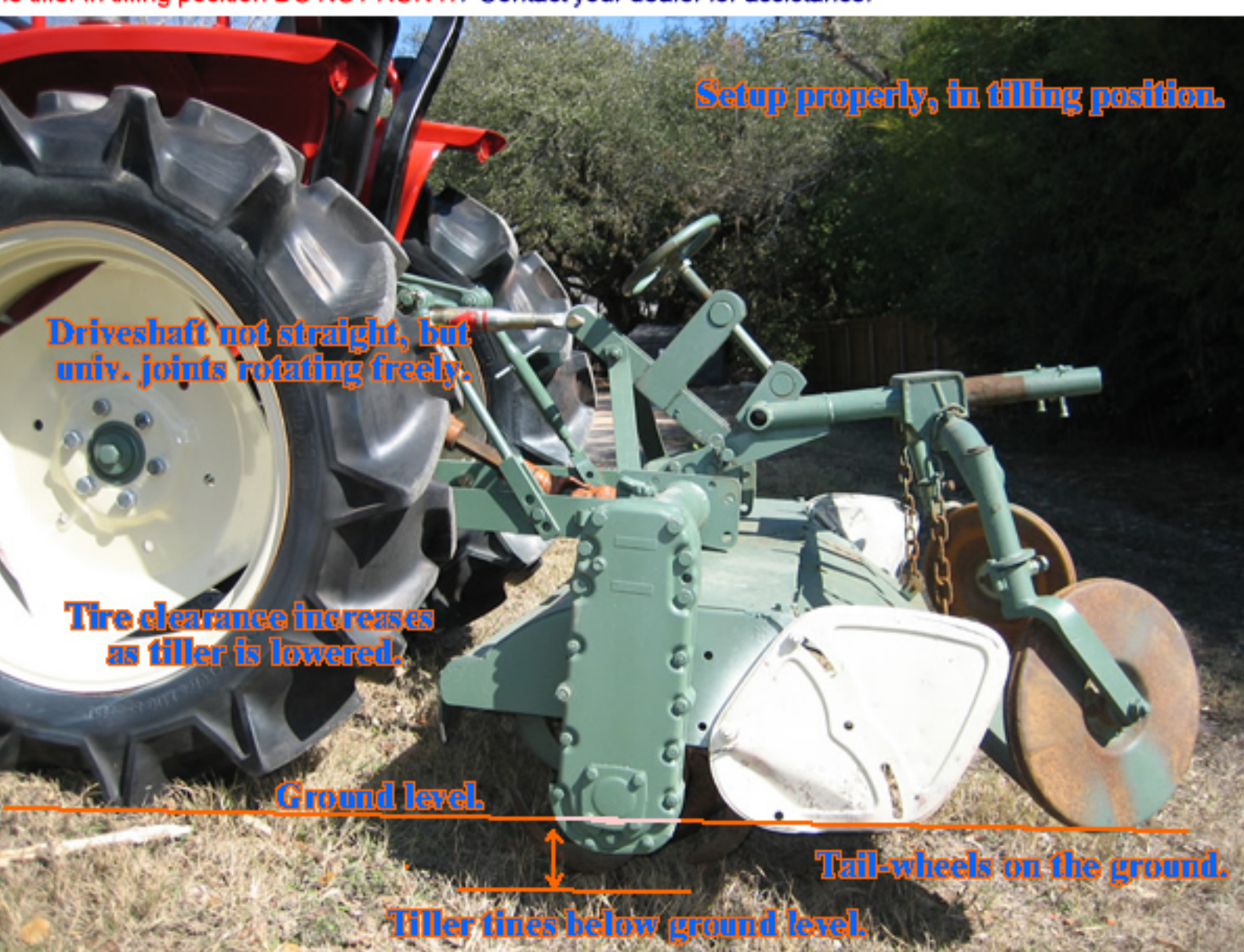
Fig. 4 shows what it will look like when you're tilling, with the tines down in the ground, and the tail wheels resting on the ground. You have to use your imagination a bit, because I don't have a good spot here at the shop to actually till. So I parked the tractor with the tiller hanging over a low spot, so that I could lower it into the actual tilling position and turn the drive shaft with the tractor shut off and the PTO in neutral. If the drive shaft binds with the tiller in tilling position DO NOT RUN IT. Contact your dealer for assistance.
