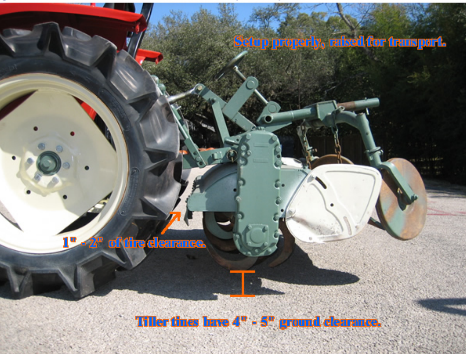
Fig. 2 shows what it should look like with the tiller raised up for transport.
